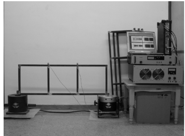
Fig. (2): The experimental setup of the frame structure.
